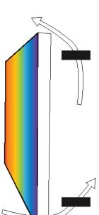
To work effectively, Cool-stick must have one opening through which room air can enter the panel's enclosure, and another through which heated air can leave. The most satisfactory arrangement is a slot of no less than 1" height running the entire width of the panel just above and just below the panel.
